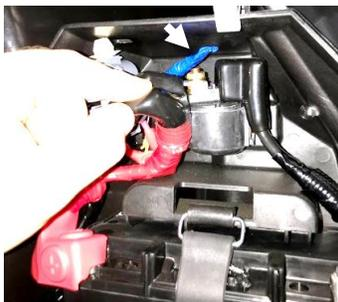
Re-torque all the fasteners after 100 miles.
