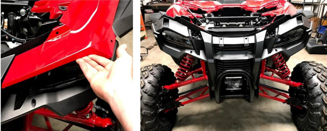
8. The bottom portion of the front fascia must now be moved to free the entire front end. Take care not to damage the bottom mounts of the fascia, or the radiator side cover shown in step six. Remove the Fascia and place it face down on a soft non-marking surface.
