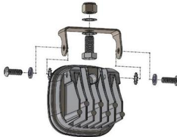
14. With the 9/16" wrench and socket, mount the lights onto the brackets as shown in the driver's side picture below. Repeat steps for the passenger side. Remove harness attached to the front fascia and set aside. It will not be reused.
